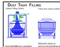
Moved to stores or process by fork lift truck and/or overhead hoist
