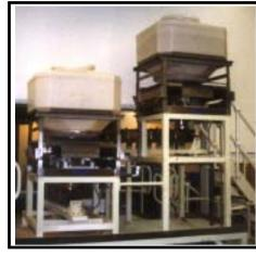
Application showing polyethylene Linkbins in a system for a major food producer
