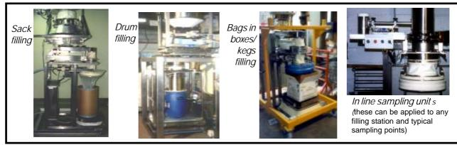
"DUST TIGHT" FIBC FILLING/DISCHARGE STATIONS (INC' WEIGHING WHERE REQUIRED).
